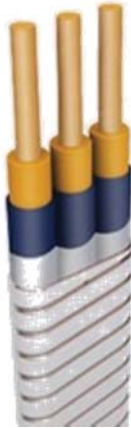
1. Conductor 2. EPDM 3. EPDM 4. F4 film 5. Nylon fabric 6. Galvanized steel tape
